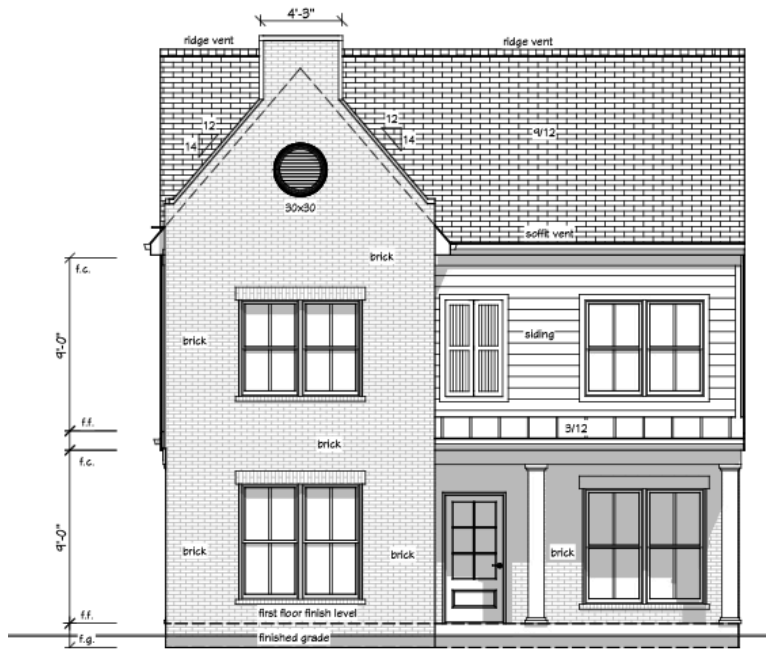
front elevation scale: 1/4" = 1'-0"
